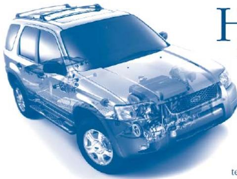
Hybrid electric vehicles (hybrids) are exciting new additions to the car market for government fleet purchases. Powered by both an internal combustion engine and a battery-operated electric motor, hybrids can achieve up to twice the fuel economy of a conventional car and produce 30 to 50 percent fewer greenhouse gas emissions. In addition to reducing our dependence on oil and improving the environment, hybrids can offer cost savings over the lifetime of vehicle ownership.
