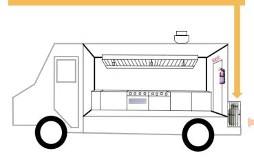
Liquified Petroleum (LP) Gas Systems ☐ 319.8.1 Maximum aggregate capacity of LPgas containers transported on a vehicle and only used to fuel cooking appliances is 200 lbs (47.3 gallons) propane capacity.
