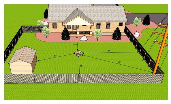
Recreational fires are **required** to be a minimum of 25' away from all combustible materials and structures, including houses, decks, fences, sheds, utility poles, etc. Other conditions which could cause a fire to spread to within 25' of a structure shall be eliminated prior to ignition. This could necessitate mowing and watering grass, trimming trees and shrubs, etc.
