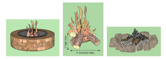
**Portable Outdoor Fireplace:** A portable, outdoor, solid-fuel-burning fireplace that may be constructed of steel, concrete, clay or other noncombustible material. A portable outdoor fireplace may be open in design or may be equipped with a small hearth opening and a short chimney or chimney opening at the top.
