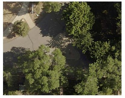
PROPOSED INTERSECTION Remove island and add pedestrian crossing with ADA ramp
